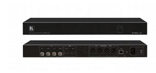
VP-475UX is a high-performance, dual channel scaler and format converter for SDI video signals of up to 12G data rate. With its integrated dual scaler, it converts the 12G SDI video signals from its two input channels (with embedded audio) to two 4K@60Hz (4:4:4) HDMI outputs, along with de-embedding the audio signals and sending them to the analog audio output ports
